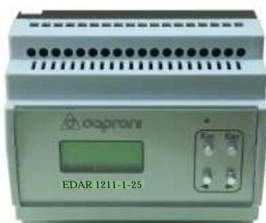
This digital amplifier EDAR 1211-1-25 is designed to control direct operated proportional directional control valves and proportional flow regulators with one solenoid without feedback.
